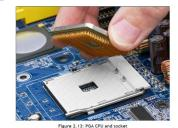
Land grid array (LGA) layouts replace the pins on the bottom of the CPU with gold pads, called lands. In an LGA, the pins are located in the pocket instead.
